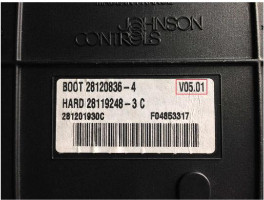
The BSI from the picture is V5.01 and can be found in vehicles from 2008 to now. The older vehicles have HW version V2.00 and are typical from 2004 to 2008.
