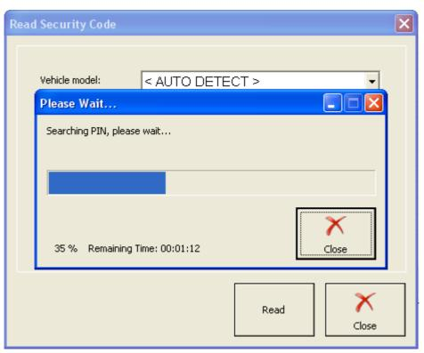
Note that PIN search always starts with checking the PIN reading capabilities that may take up to 15 minutes. Some BSI's require some additional specific operations to be performed – this is "Working on BSI" phase – up to 5 minutes. At the end the following message should appear:
