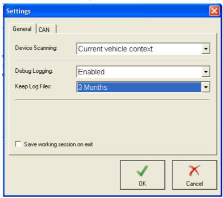
Device scanning: "Current vehicle context" search units only specific for the currently selected vehicle, "All devices/on CAN/on K-Line" search available units in all possible units.
