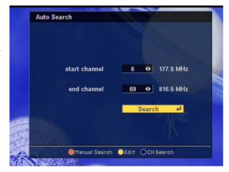
Receiver will automatically search the channel for TV and Radio, during this procedure you can see the already scanned in channels in the Auto Search Page on screen.
