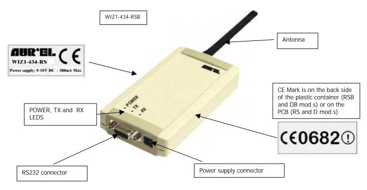
The WIZ1-434-x modules are half-duplex, smart transceivers that support a digital data packet transfer of 1-120 bytes length at 9600 b/s speed. The data transferred to the remote unit are error-free since at the arrival are verified and confirmed.
