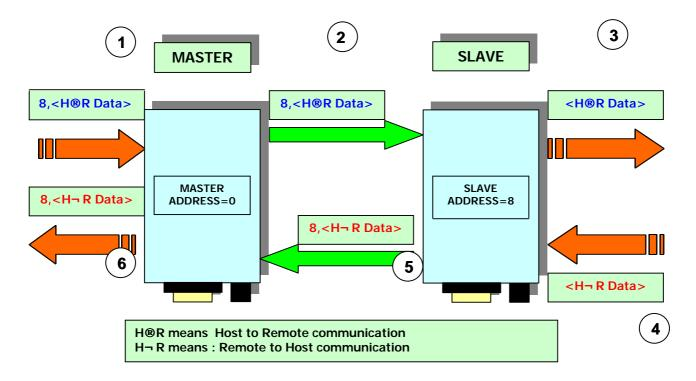
**1.** Data addressing is managed by the system placed upstream of the WIZ1 master module: the address byte of the remote WIZ1 module, is placed before the data packet byte.
