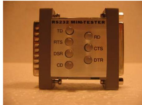
This mini RS-232 Tester will allow you to watch transmit (TD) and receiver (RD) data traffic.
