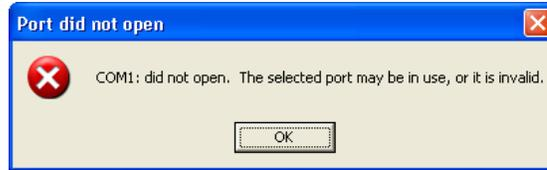
This normally indicates some other application has control of the port and needs to be shut down. Most often the culprit is the HotSync Manger in Palm Desktop used to hot sync the Palm Pilots. This is recognized by the HotSync icon in the computers task bar. Right hand click and select “Exit” to shut down this application and free the port for use by Elite Wireless.
