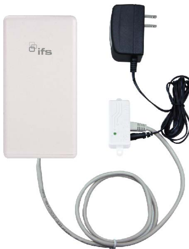
Figure 3-4 Connect the PoE injector
