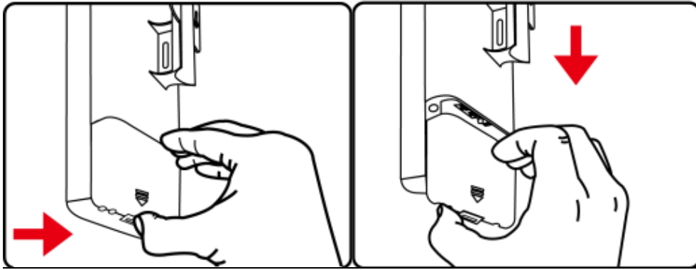
Figure 3-1 Connect the Antenna
