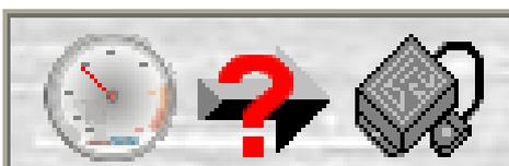
**Program MicroTHERM Warning:** Channel data has been altered (in the setup screen) but the MicroTHERM control unit has not yet been reprogrammed with this new data. This programming must be done to update MicroTHERM or it cannot carry out the control as you require!
