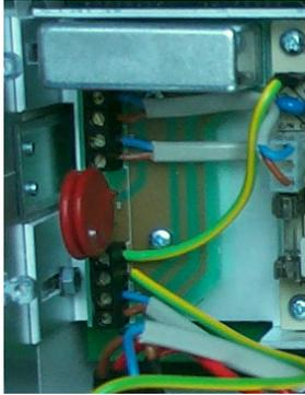
Figure 54 Varistor & Filter Unit
