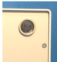
Figure 56 Battery Connector
