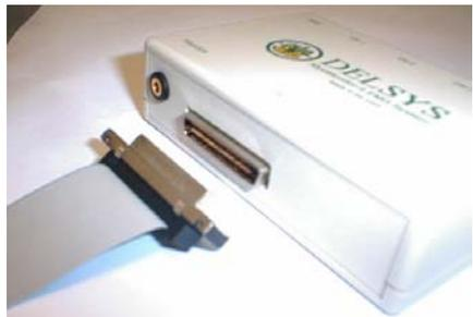
Figure 1: Connecting the A/D card in the Jornada and the Interface Unit. Follow the instructions above.
