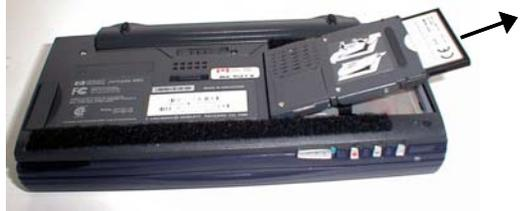
Figure 8: Removing the CompactFlash Memory Card. Follow the instructions above.
