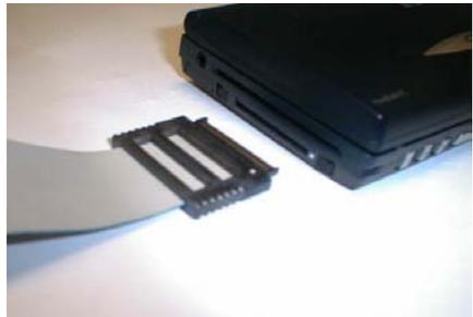
2. Connect the SCSI connector end of the A/D cable into the I/O jack on the back of the MyoMonitor Interface unit.
