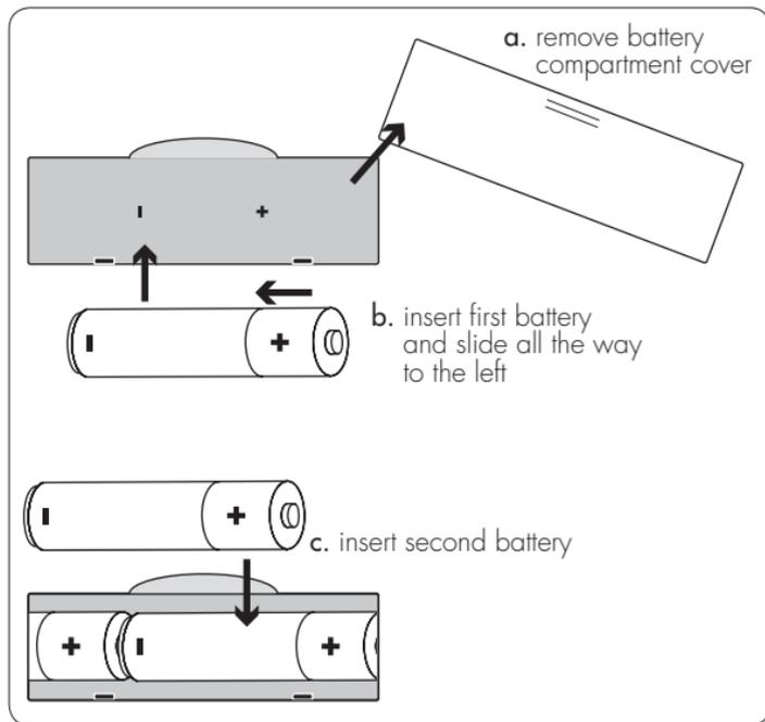
2. Insert 2 AAA batteries into the mouse battery compartment.
