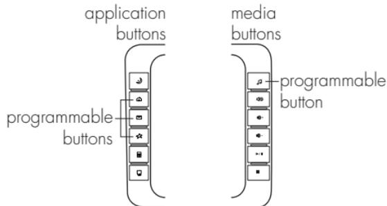
► **note** You can change the functions of the four programmable buttons on the keyboard to launch a variety of programs. The remaining multimedia and application buttons on your keyboard are pre-programmed with default settings (shown in “your new keyboard” on page 3) and cannot be changed.
