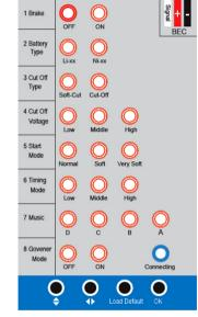
3. Connect the power pack to ESC;
