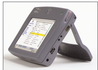
Side Interfaces – RS-232C serial port, USB port, microphone and headphone jacks, Kensington lock (opposite side).
