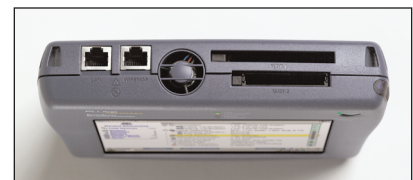
Top Interfaces – 10/100/Gigabit port, wire map port, CompactFlash® and PCMCIA slots.
