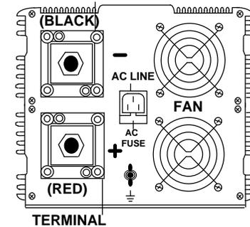
CAUTION : DO NOT REVERSE INPUT. USE RED BATTERY CORD TO CONNECT (+) OF A DC BATTERY TO (+) TERMINAL. AND THEN, USE BLACK BATTERY CORD TO CONNECT (-) BATTERY TO (-) TERMINAL.
