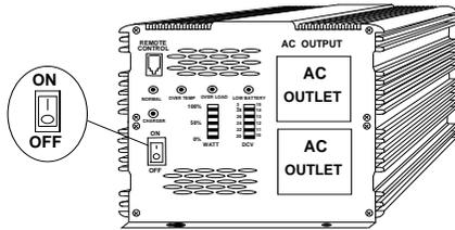
**STEP2: WHEN CONNECTED TO ANY APPLIANCE, BE SURE TO TURN ON INVERTER FIRST. AND THEN, TURN ON THE POWER SWITCH OF THE APPLIANCE.**
