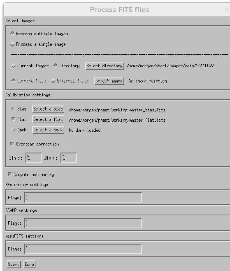
Figure 4.3: PhAst’s batch processing allows for the calibration of an entire directory of files, or all currently loaded files.
