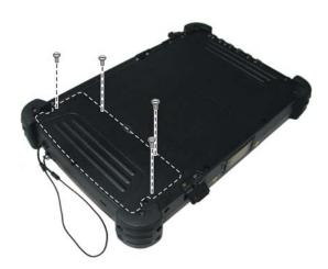
4. Fit the battery pack into place  $(\mathbf{0})$  and secure with two screws  $(\mathbf{2})$ .
