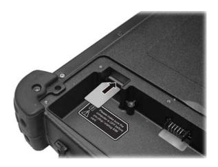
To remove the SIM card, just push in  $(\mathbf{0})$  the SIM card to pop-out  $(\mathbf{0})$  and remove the card.
