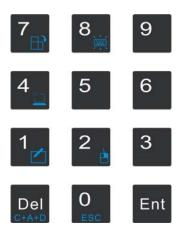
When the **Fn** keylock is ON ( **m** icon appears on the system tray), you can use the following secondary functions with blue color on top of each button.
