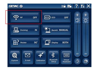
Click the RF button to switch the WLAN radio on/off, indicated by the WLAN indicator ( ) glowing in green when on.
