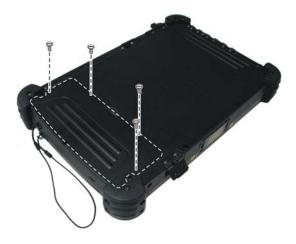
4. Remove the two screws securing the battery pack to the battery compartment (①) and, pull on the ribbon strip to lift the battery pack off the tablet PC (②).
