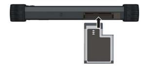
3. When a new card is seated, the tablet PC will detect it and try to install the appropriate driver. Follow the on-screen instructions to complete the process.
