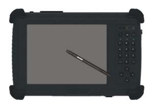
**WARNING:** To protect the LCD screen with active digitizer feature, do not use force when pressing on the surface (greater than 1 kg and more than 30 seconds at a time).
