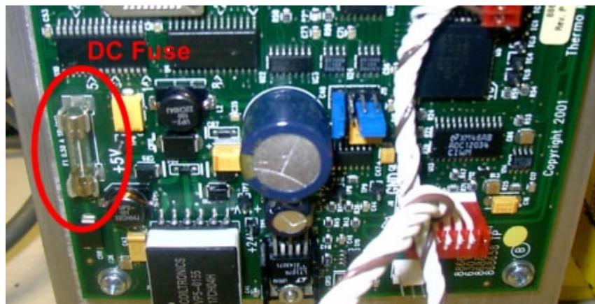
**Figure 11–3.** Fuse on CPU board for gauges with DC power
