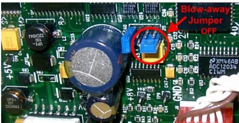
**Figure 11–9.** Blow-away jumper in normal operation position
