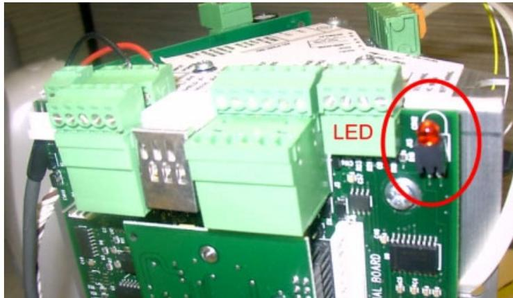
**Figure 11–1.** Power LED on the CPU board
