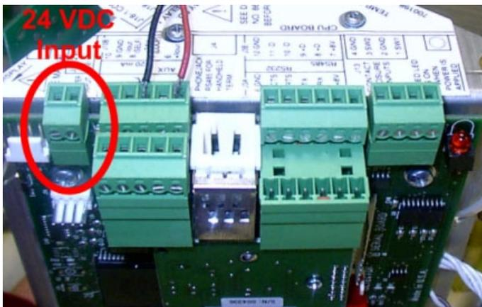
Figure 11–4. J12 connector on the CPU
