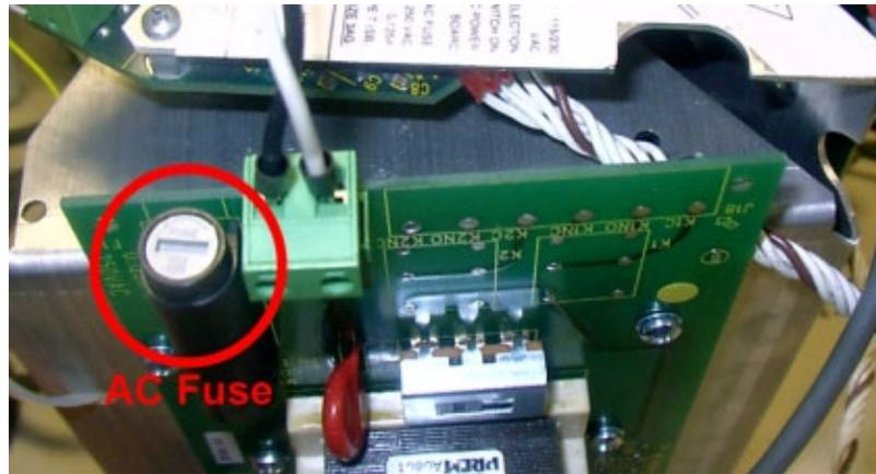
**Figure 11–2.** Fuse on AC power supply board
