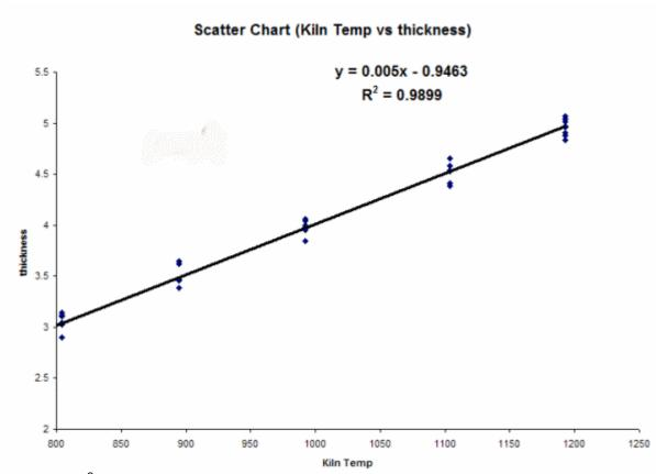
The high R<sup>2</sup> value indicates that the model is a good fit. As the Kiln temperature increases, so does the thickness.
