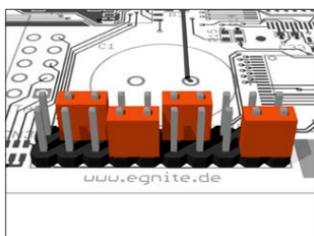
**CPLD JTAG** Routing the JTAG interface to the CPLD is provided by shortening pins 2 and 4, 7 and 9, 12 and 14 as well as pins 15 and 17. Note, that you need a special Xilinx adapter for programming the CPLD via JTAG.
