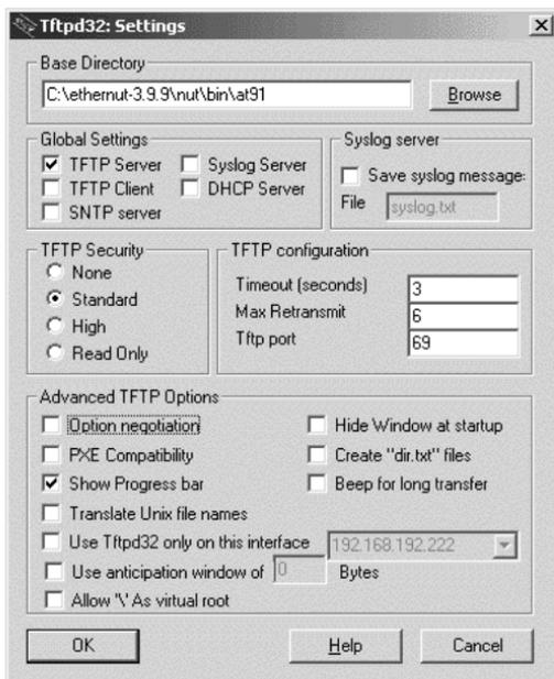
After pressing the reset button, BootMon will request the binary image from the TFTP server running on your PC. On TFTP32 the following should appear.
