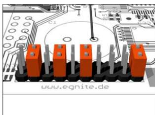
**Internal JTAG** As an alternative, the Ethernet is able to program its own CPLD. The required jumper configuration is shown on the left. This configuration may be combined with the first one (CPU JTAG), in which case you can download the CPLD programming software to the CPU via JTAG. As soon as this software starts running, it will program the CPLD.
