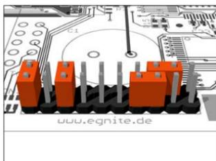
**CPU JTAG** Jumper JP5 routes the JTAG signals to the AT91R40008, if pins 3 and 5, 8 and 8, 15 and 16 as well as pins 19 and 20 are shortened. This is the default configuration and is used to upload software to the CPU or burn the FLASH Memory.
