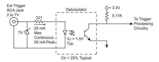
Figure 78. External Trigger Input Circuitry
