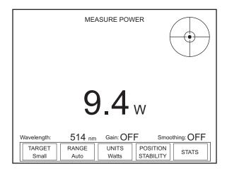
Figure 12. MEASURE POWER: Thermopile Quad Sensors
