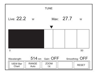
Figure 31. TUNE: Bar Chart (Thermopile and Optical Sensors)
