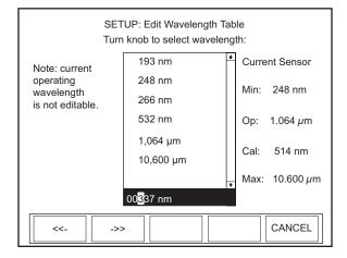
Figure 56. SETUP: Edit Wavelength Table (Adding a Wavelength)
