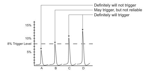
Figure 19. Internal Trigger Threshold
