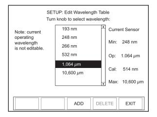
Figure 55. SETUP: Edit Wavelength Table
