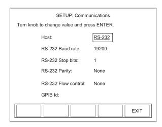
Figure 63. SETUP: Communications (Changing the Values)
