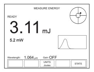
Figure 16. MEASURE ENERGY: Thermopile Sensors (Long Pulse - After Pulse)
