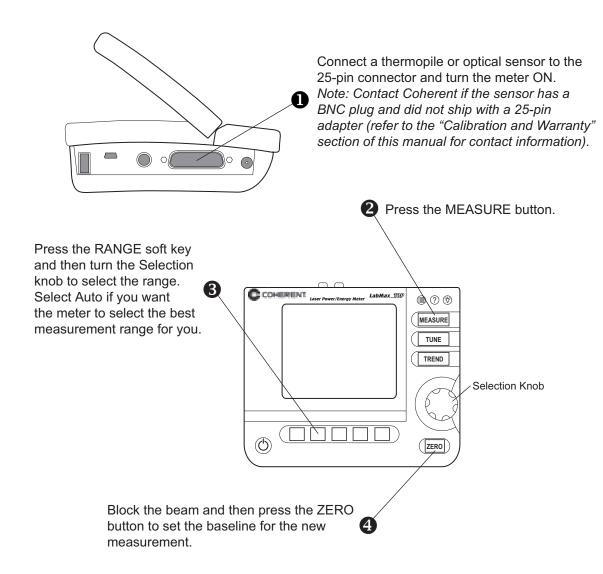
**5** Unblock the beam, take the measurement, and observe the result on the display.
