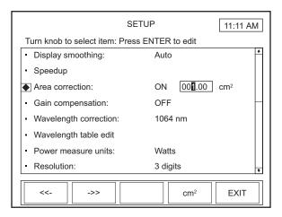
Figure 51. SETUP: Area Correction
