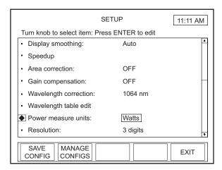
Figure 57. SETUP: Power Measure Units
