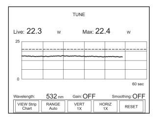
Figure 30. TUNE: Strip Chart (Thermopile and Optical Sensors)
