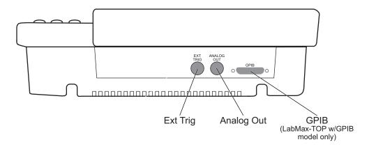
Figure 9. Rear Panel Connectors
