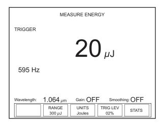
Figure 17. MEASURE ENERGY: Pyroelectric Sensors
