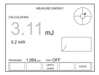
Figure 15. MEASURE ENERGY: Thermopile Sensors (Long Pulse - Active)
