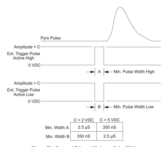
Figure 79. External Trigger Minimum Pulse Width
