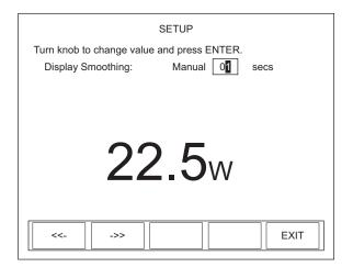
Figure 48. SETUP: Display Smoothing (Thermopile and Optical Sensors - Manual Mode)
