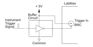
Figure 80. Boosting Source Current of Triggering Device
