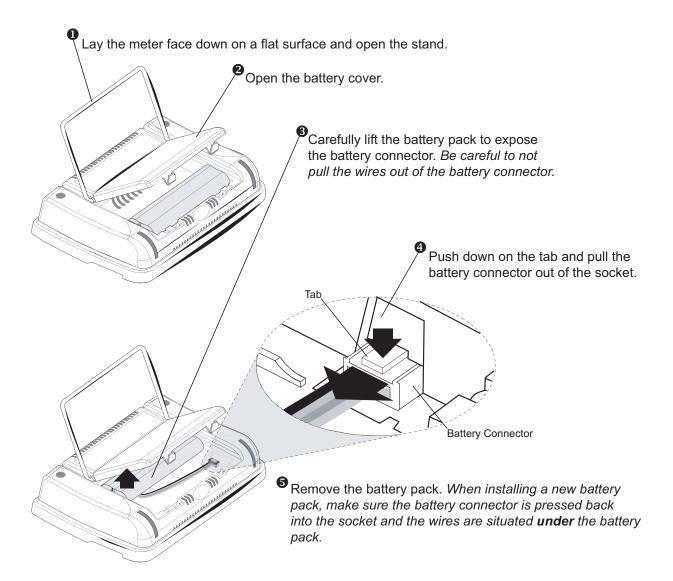
Figure 10. Battery Pack Replacement
