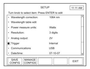
Figure 60. SETUP: Trigger
