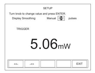
Figure 49. SETUP: Display Smoothing (Pyroelectric Sensors - Manual Mode)
