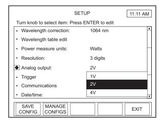
Figure 59. SETUP: Analog Output
