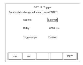
Figure 61. SETUP: Trigger (Changing the Values)
