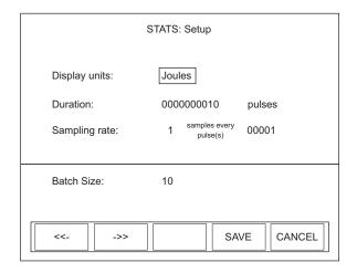
Figure 27. STATS: Setup (Pyroelectric Sensors - Energy)
