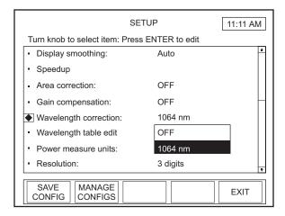
Figure 53. SETUP: Wavelength Correction
