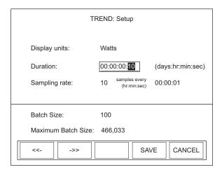
Figure 44. TREND: Setup (Thermopile and Optical Sensors)
