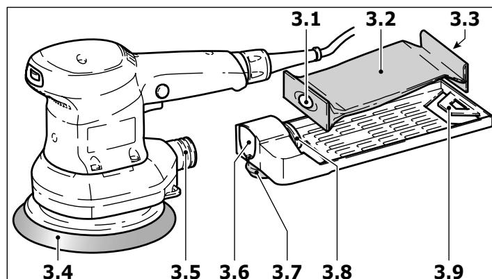
The machines are fitted with inbuilt extraction as standard. The sanding dust is extracted through suction openings in the sanding base (3.4) and trapped in the turbo-filter (3.2).
