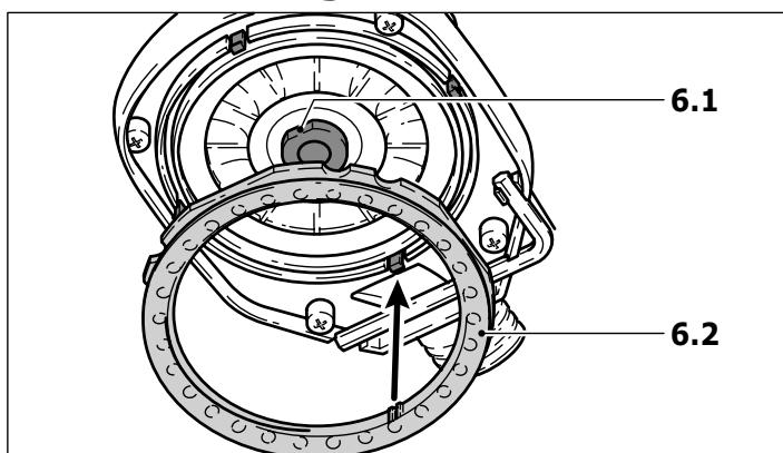
The sanding base is braked by a collar (6.2) in order to prevent any uncontrolled excessive speed of the sanding base. Because the collar wears down in the course of time, it has to be replaced by a new one (453388) as soon as there is any reduction in the braking effect.
