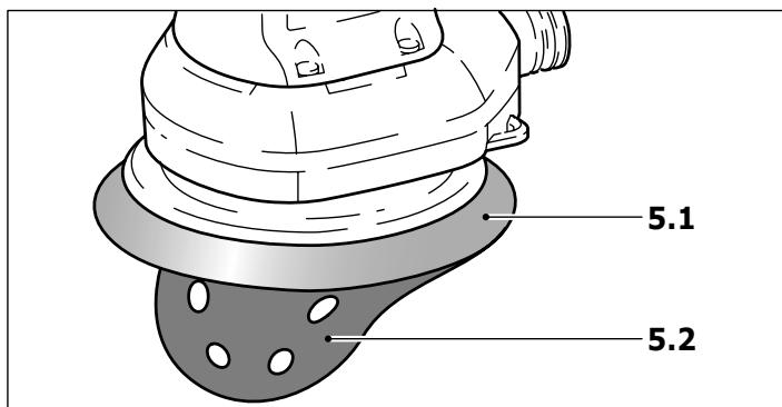
The self-adhesive sanding material (5.2) is simply pressed onto the sanding base (5.1) and held safely in place by the Stickfix sanding base velcro surface.
