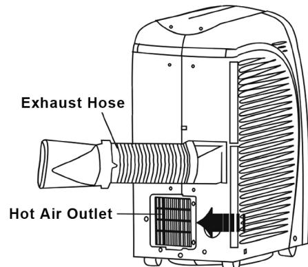
The hot exhaust air can be vented through the wall or out a window. If mounting in the wall, the height of the hole should be 16 to 50 inches (40cm to 130cm).
