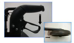
3) To lock the brakes push down both brake levers at the same time until they lock. To unlock pull up brake levers until the lock disengages.
