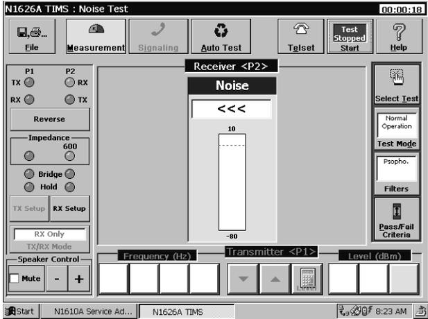
**Note:** The Transmitter **Frequency** and **Level** controls are not available since the Noise test is conducted in RX-only mode.
