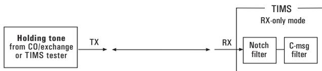
Signal-to-Total Distortion with Holding Tone
