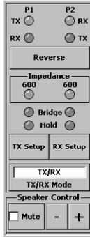
The TX/RX setup controls on the left side of the screen configure the TIMS line connector ports (P1 and P2).
