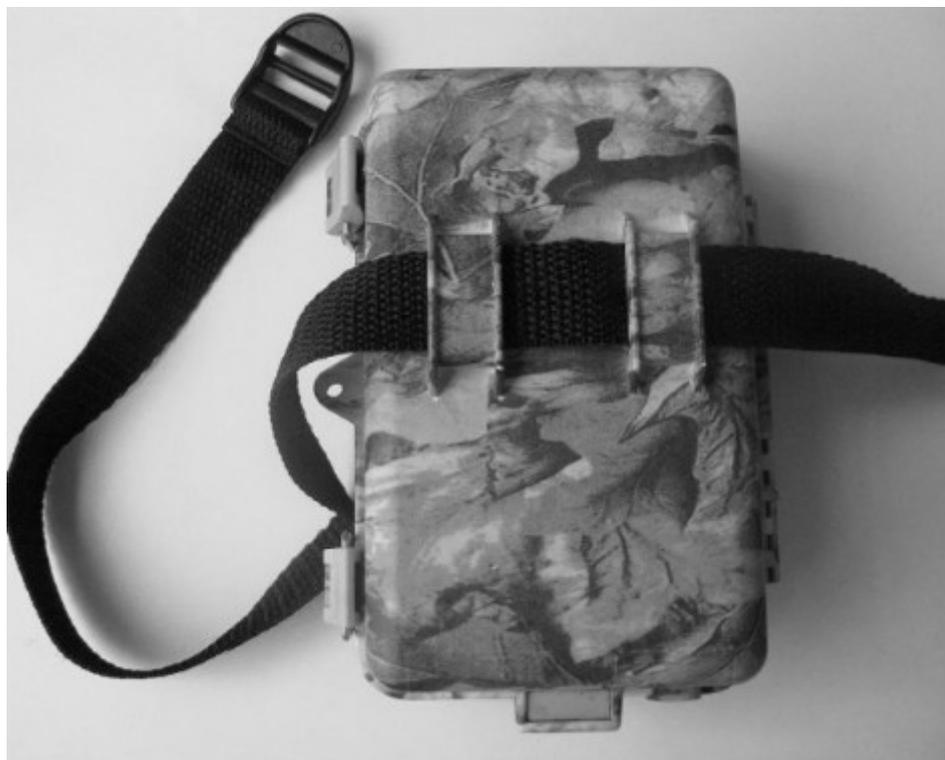
Figure 4: Fixing the camera with belt
