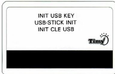
**Re-initialisation with the Time Recorder unit can only be performed with the INIT USB KEY badge on units from serial number 05N6, and onwards**
