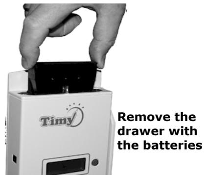
**Remove the drawer with the batteries**
