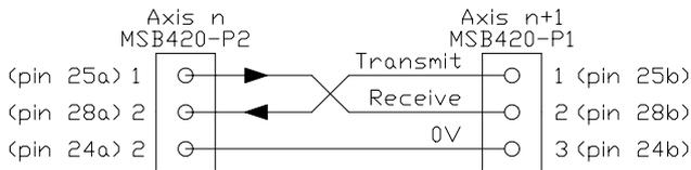
As the RS232 signals are a true *daisy-chain*, if a card is removed in a multi-axis system, the connection to subsequent axes will be lost.
