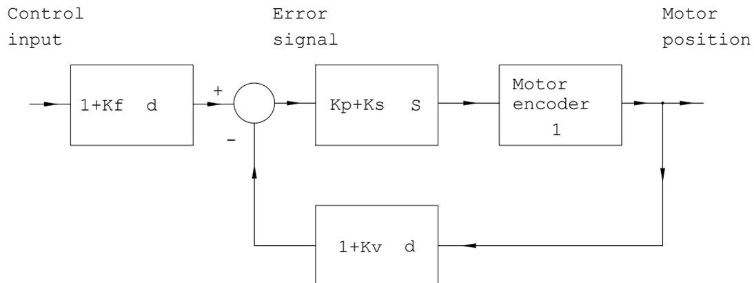
The above diagram illustrates the relationship between the control coefficients in a PM304 servo loop. The *control input* is a number generated by a move command.
