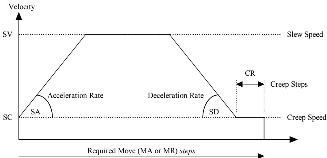
The end of a move is defined as having occurred when the actual position has settled close to the required position. The distance at which the motor starts to *settle* is set by the **WI** (end of move window) command. For the move to be defined as being complete, the motor must *settle* within the end of move window for the time set by the **SE** (settle time) command.
