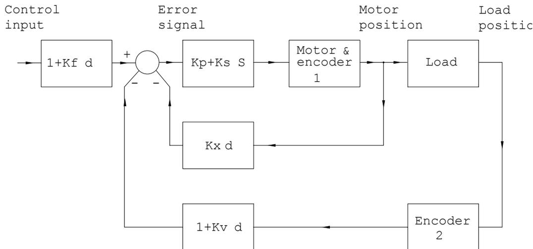
The increased resilience of the coupling between Encoder 1 and the motor compared with that of Encoder 2 means that the value of **KX** may be much larger than **KV**
