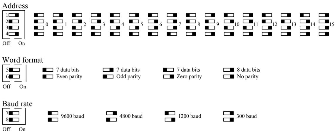
The above example shows a controller set to axis 9 with communications at 9600 baud, 7 data bits and an even parity bit. There is always one stop bit.
