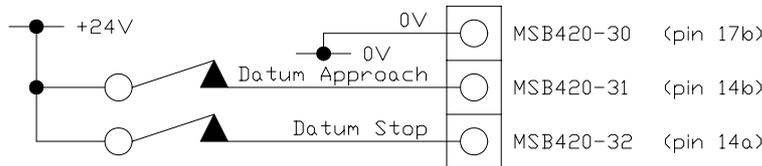
The switches should be positioned so that they are activated as the load passes them and will therefore not be damaged.
