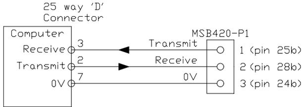
Connections for PM304s in multi-axis applications:
