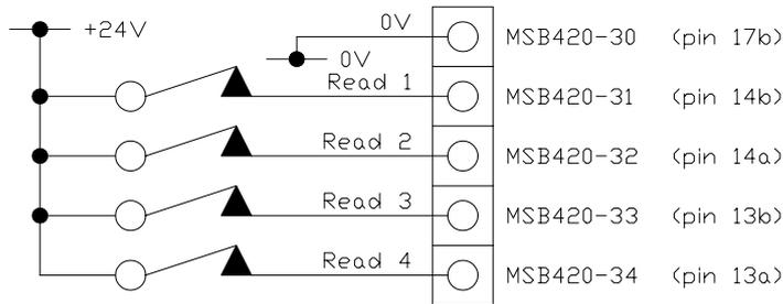
The **RP** Read input Port command is used to check the operation of the *read ports*. This instruction returns a four digit binary number of either **0** or **1** characters to represent the current state of the read port. These start with read port 4, through to 1. Referring to the diagram above, a **0** represents a switch closed and a **1** represents a switch open.
