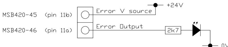
The Error output is typically used in a system to disable the Servo amplifier such as the DCD60 series.
