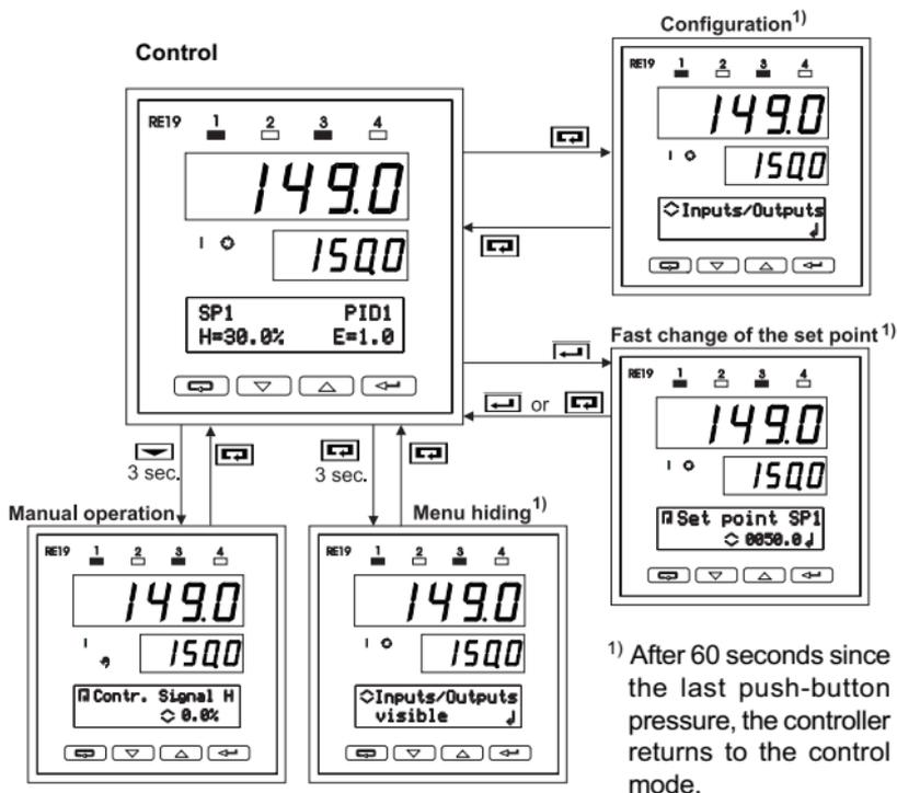
**Fig.4.2. Transition diagram between controller operation modes**
