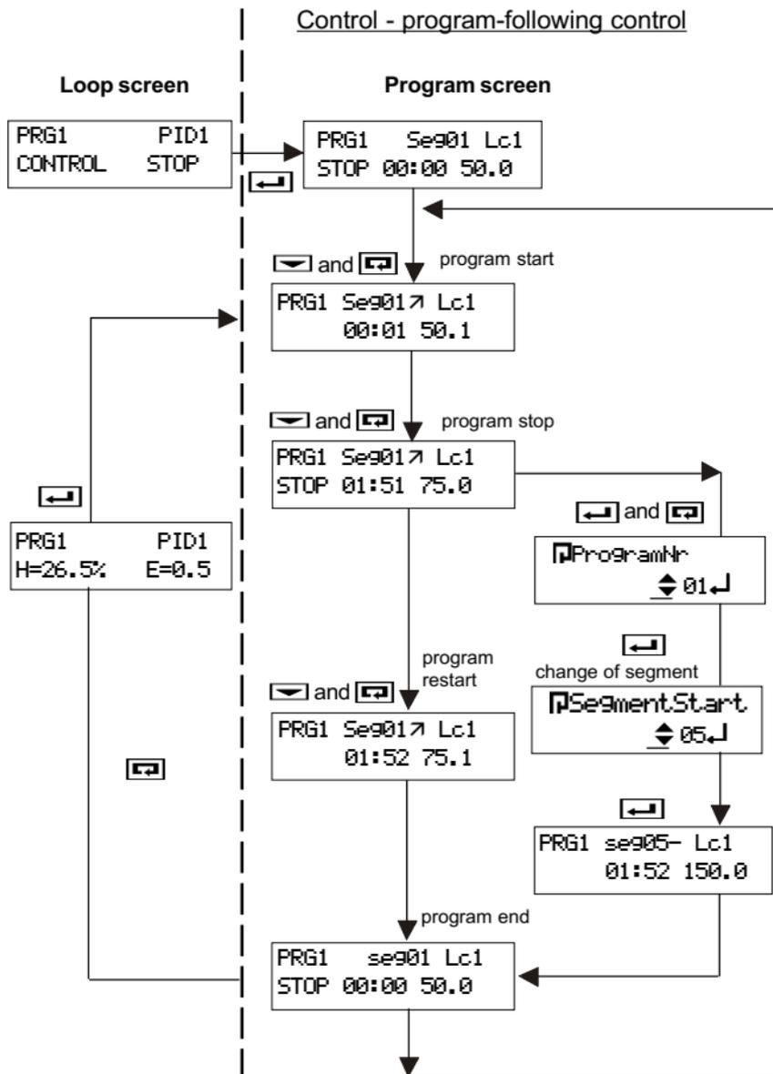
**Fig.8.4. Example of program operation control**
