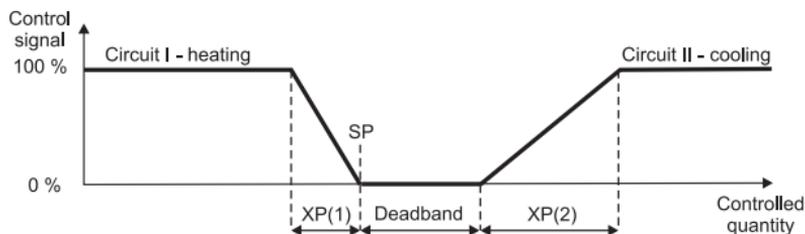
**Fig.7.1. Control with two heating-cooling circuits**
