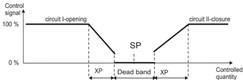
**Fig.7.2. Valve control**
