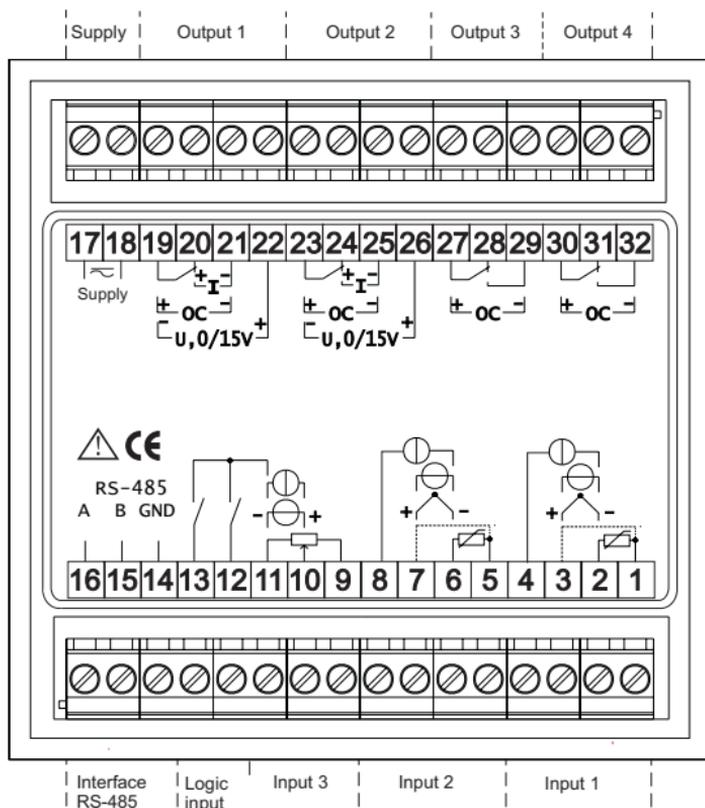
**Fig.3.3. Description of the terminal strip.**
