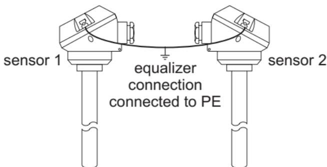
**Fig. 3.1. Connection of two sensors.**
