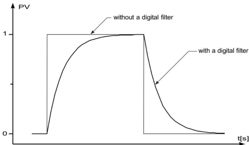
**Fig.6.1. Time characteristic of the filter.**
