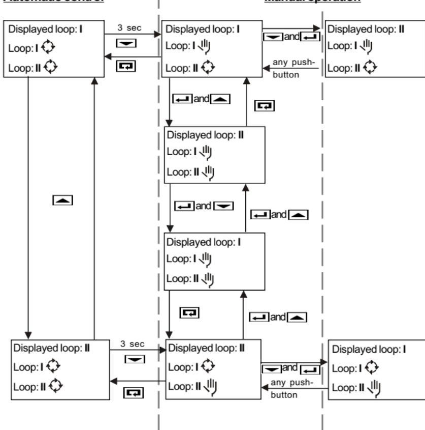
**Fig.4.3. Manual control diagram**
