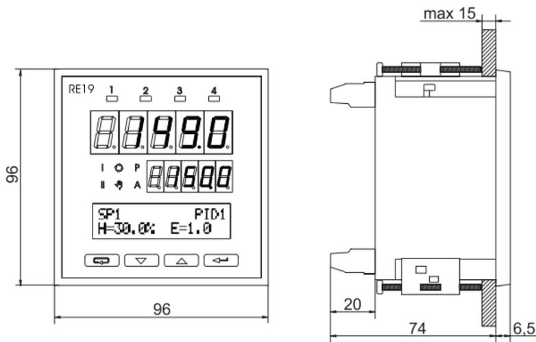
**Fig. 3.2. Controller overall dimensions.**
