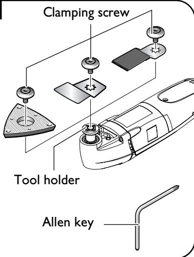
**Attaching/replacing the sanding sheet (Figure 5).**
