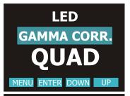
**GAMMA CORRECTION** Linear = Linear current output Quadratic = Linear light output (default)
