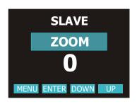
The SLAVE unit receive DMX signal from the MASTER unit. By setting all the SLAVE units connected to the MASTER, to DMX address 1, them will be synchronized with the Master unit following the chase selected on it, but running their own Pan&Tilt and Zoom position.
