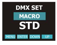
**MACRO** STD = Standard mode enabled EXT = Extended; enable rainbow effects on Macro channel (DMX ch 16)
