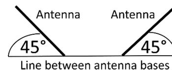
**NOTE!** Do **NOT** bend antennas backwards over the module; doing so will cause poor performance and may cause undesirable out-of-band radio transmissions.
