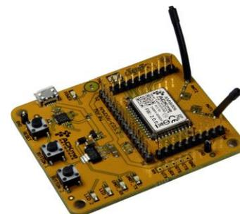
Figure 9 - AMW006-E03 eval board with wire antennas
