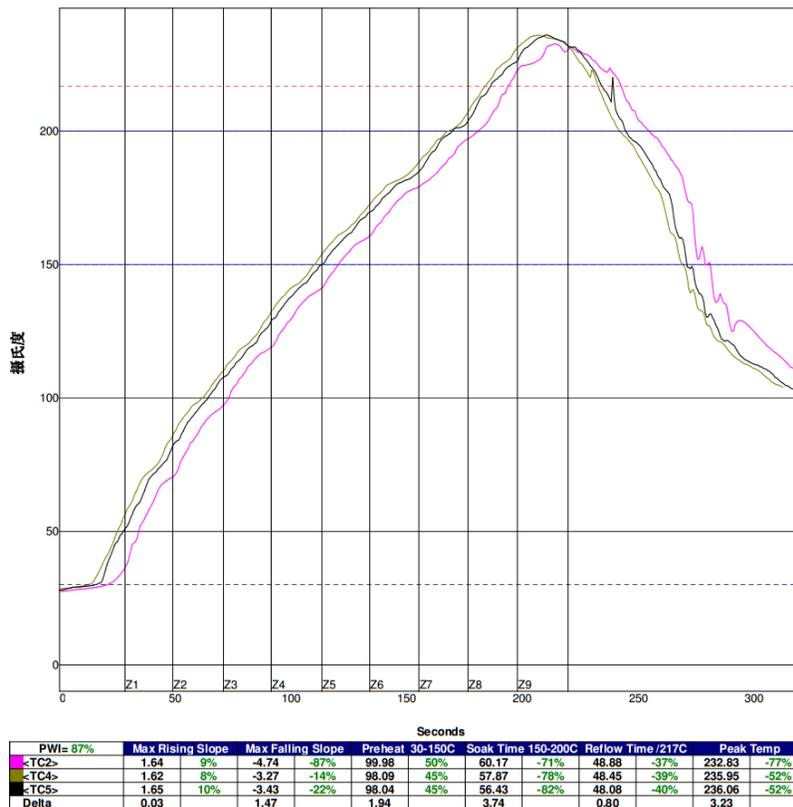
Figure 6 - Example solder reflow profile (AMW006-E03 evaluation board)
