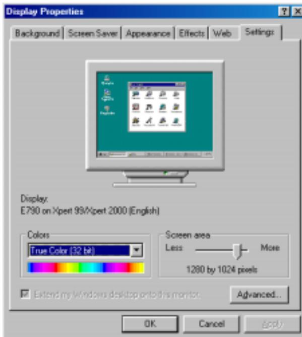
Locate the area on the Display Properties box labeled Desktop Area. The slide bar in this area is used to adjust the screen resolution. The current resolution will be displayed below the slide bar. The resolution must be set to a minimum of 1024 by 768 or portions of the DataLink tool bar will not be visible. We recommend a setting
