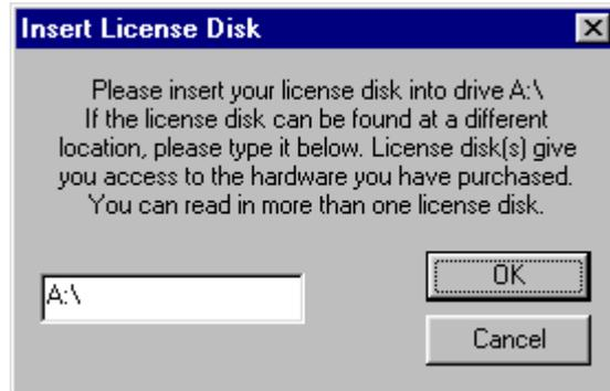
Insert the license disk into the floppy disk drive, type the correct drive letter in the dialog box and select **OK**.
