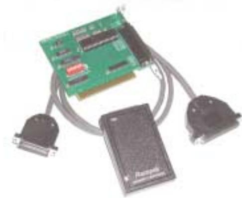
The PIO-12 board requires an available ISA expansion slot in your PC. Before proceeding insure that your PC has an available ISA slot. Some PC's only have PCI expansion slots and cannot be used with the PIO-12 expansion board.
