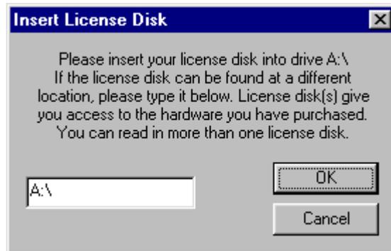
Insert the license disk into the appropriate drive. Enter the corresponding drive and select OK to copy the license information
