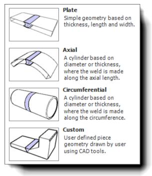
When Axial is selected the default Plate piece graphics are removed and replaced with Axial piece graphics.
