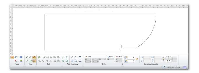
Now we will trace in the internal targets from the bitmap onto our piece. We will use the 💿 Draw Piece Circle tool found in the Add Geometry section of the CAD Toolbar to trace our targets.
