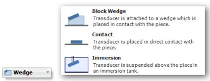
Changing the wedge mode will remove the wedge display from the drawing pane and will automatically set a new default value for the probe's elevation offset.
