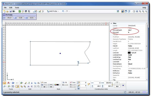
Select the outline with the 100mm radius, and In the Geometry Inspector Set ExtrudeZ to 12.7 and ExtrudeDepth to 12.7
