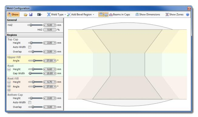
To modify the bevel configuration, pre-defined weld bevels can be selected from the **Weld Type** drop-down, specific bevel regions can be added to the weld via the **Add Bevel Region** drop-down, and regions can be configured via the **Regions** panel.
