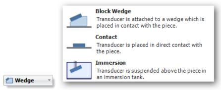
Changing the wedge mode will remove the wedge display from the drawing pane and will automatically set a new default value for the probe's elevation offset.
