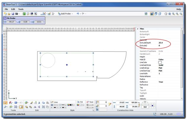
Add the Side Drilled Holes and Lucite Insert into the drawing. Set their ExtrudeZ to 0 and the ExtrudeDepth to 25.4
