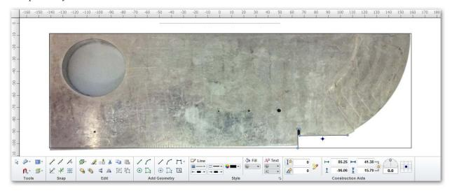
Click on the  $\Pi$  Snap Settings icon found in the Tools section of the CAD Toolbar. Click on the  $\checkmark$  Snap to Nearest icon to avoid gaps while tracing.
