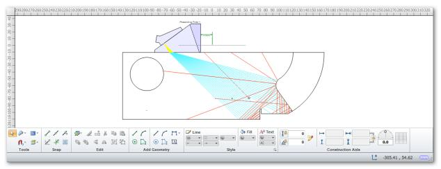
If we don't want the beamset to interact with the 50mm radius we can right click on each of the lines we used to create it and turn Reflective off by removing the check mark.
