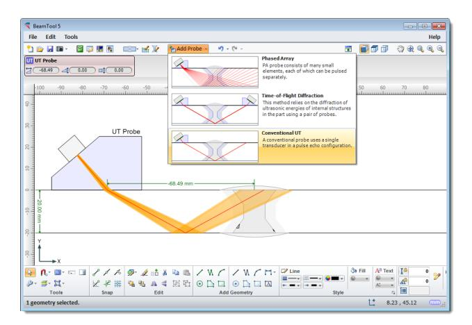
Open the UT Probe Configuration menu by clicking on the  $\swarrow$  Probe Config icon found in the UT Probe menu. Turn off the Show Beam Spread by clicking on the  $\triangleright$  Show Beam Spread icon. Detecting reflections requires that the probe/beamset is configured with enough beam skips to allow the beams to return to the transducer. Change the number of beam skips to 4 by clicking on the  $\bowtie$  Beam Skips icon.
