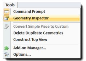
Select the 50mm radius outline, and in the Geometry Inspector set ExtrudeZ to 0 (this is the starting point of the geometry in the Z axis), and ExtrudeDepth to 12.7 (This is the depth the Geometry is Extruded)
