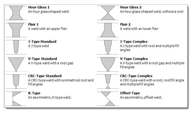
These pre-defined weld types have been constructed with regions that have been customized to particular real-world weld bevel types. Once a pre-defined weld has been selected, its regions are displayed in the Regions Panel.
