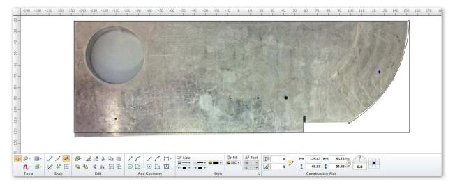
With all the outside edges of the bitmap in place we will select the rectangle and right click on it. Select Convert Selected to Lines from the dialog box. This will allow us to manipulate each line of the rectangle.
