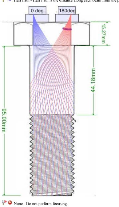
Pr Malf Path - Half Path is the distance along each beam from the point where the beam enters the piece.
