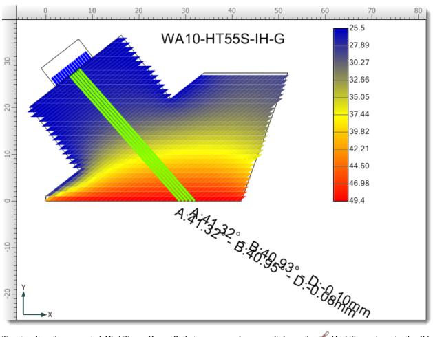
To visualize the corrected HighTemp Beam Path in your workspace, click on the  $\checkmark$  HighTemp icon in the PA Probe Configuration dialog box. When turned on, the original beam path is greyed out, and the HighTemp beam path is shown in bold.
