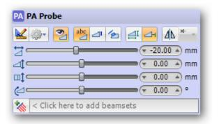
The <u>Probe Configuration</u> dialog box has many attributes that can be set for that type of probe. To specify a value you can a) move the slider right or left, b) click the right or left value spinner or c) click on the value displayed in the value spinner and type a value. The preview and drawing panes will update on the fly as the values are modified.
