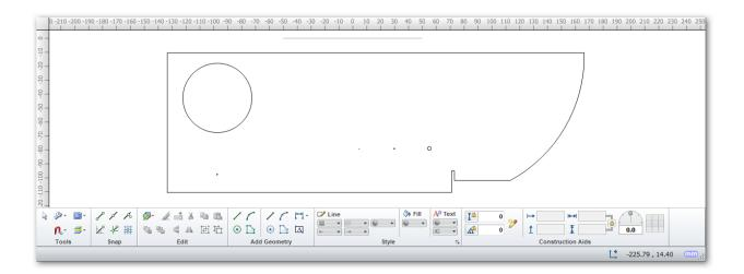
Now we will trace the 50mm radius using the C Draw Piece Arc and the C Draw Piece Line. These can found in the Add Geometry section of the CAD Toolbar.
