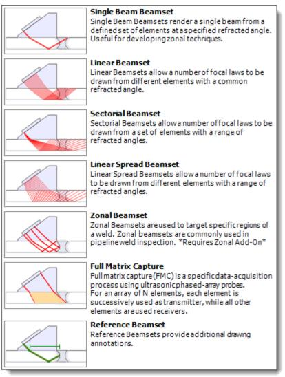
Beamsets can be <u>added</u> to a phased array probe by clicking the **\* Add Beamset**, or one of the seven beamset icons on the appropriate probe group.
