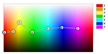
When configuring Phased Array beamsets Color List can be selected from the Beam Type picklist and the colors specified for Beam Skip Coloring are applied to the beam. If the number of 1/2 beam skips displayed exceeds the number of colors specified for the Beam Skip Coloring the color order is repeated.
