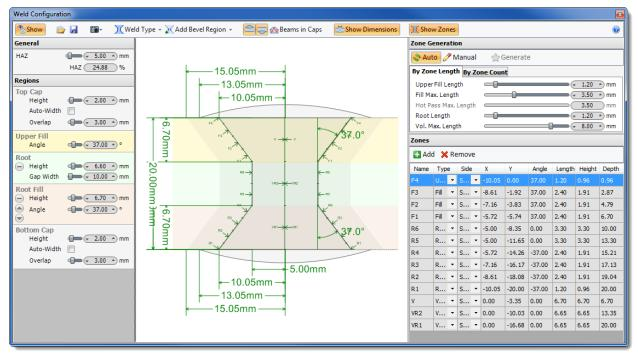
Weld Zones are constructed from the <u>Weld Regions</u> defined during the weld configuration. As a weld bevel is configured, <u>Weld Regions</u> are automatically divided into Weld Zones using the related zone configuration parameters.
