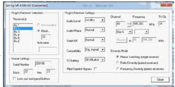
Example: Right click on the receiver display in the VR panel, and then select "Set Up VR" to get the screen above to select the transmitter groups.
