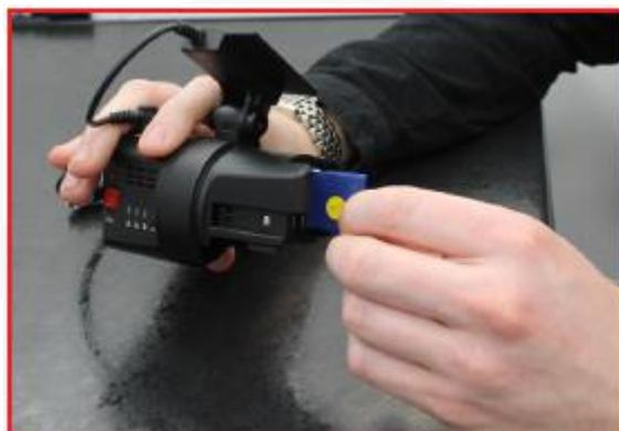
If you are using a 3G/4G USB dongle you will also need to ensure that this is inserted before you power on the unit.
