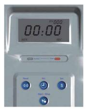
The Reset button is used to clear parameters.
