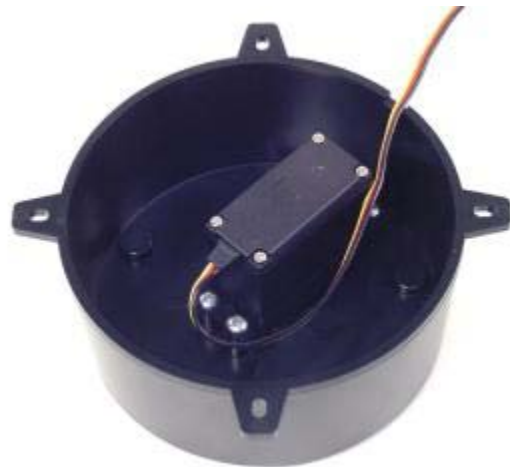
Figure 6. Servo Base Installation
