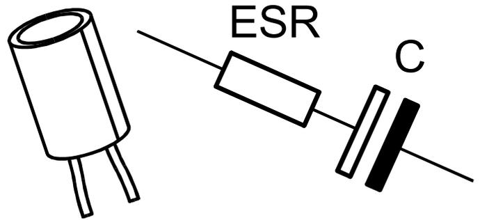
No capacitor is ideal of course, the detailed equivalent circuit of a typical capacitor is very complex. For many electrolytic capacitors however, the most important parameters regarding the capacitor's performance is the capacitance and the ESR.
