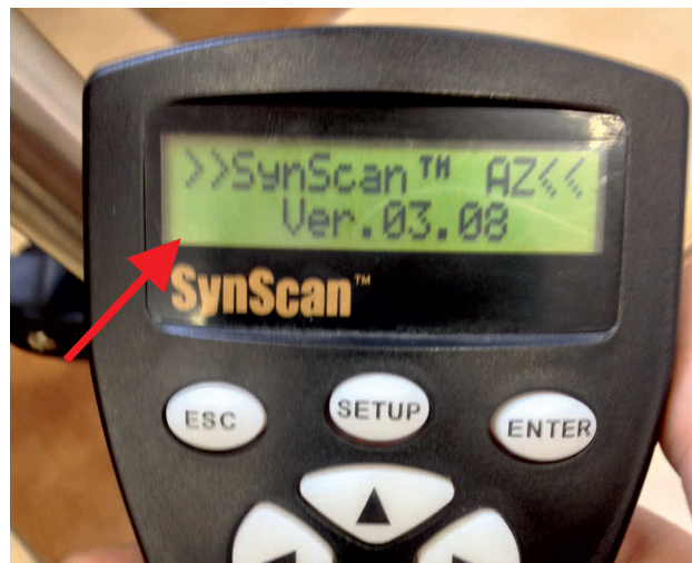
18. If both cables are connected properly, the hand controller starts operating. A beep will notify you of this
