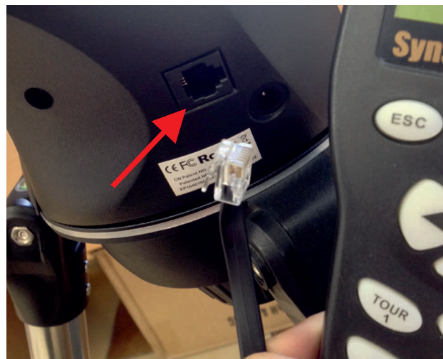
16. RJ-4 connector of the hand controller cable goes into the mount
