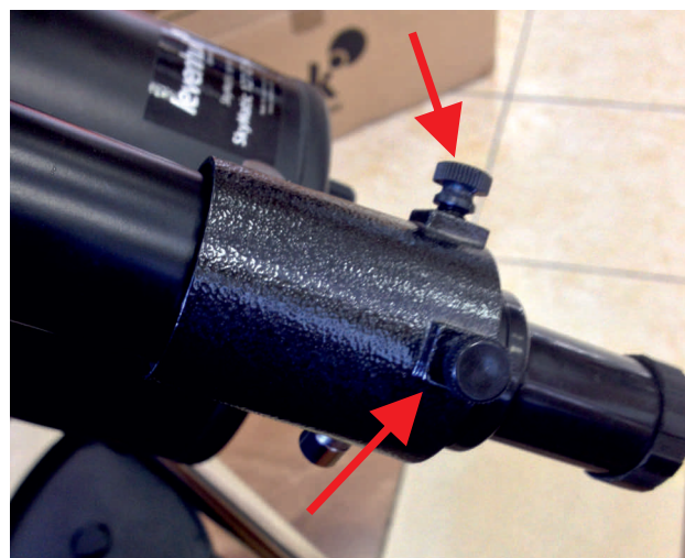
10. Adjustment screws for alignment of the optical axis
