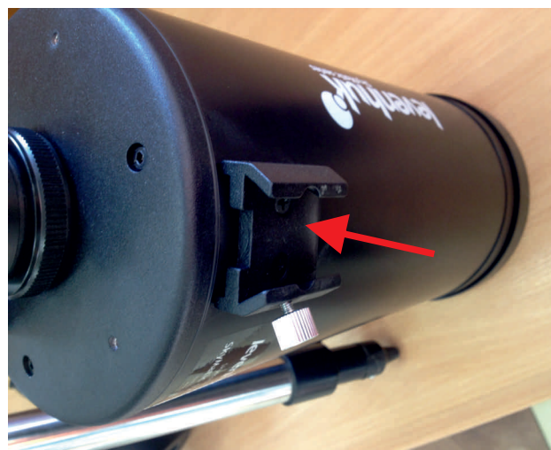
8. Dovetail plate on the optical tube
