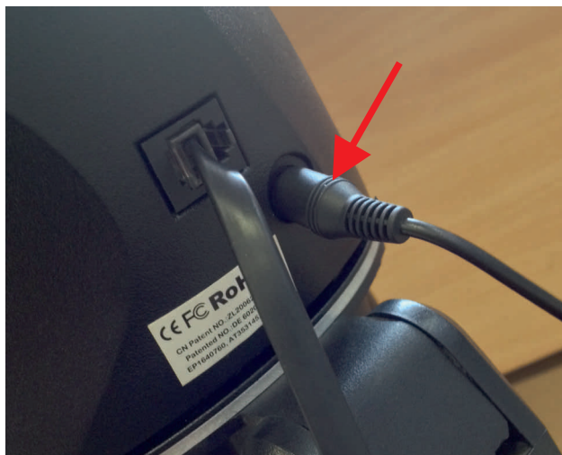
17. Power cable connected to the mount
