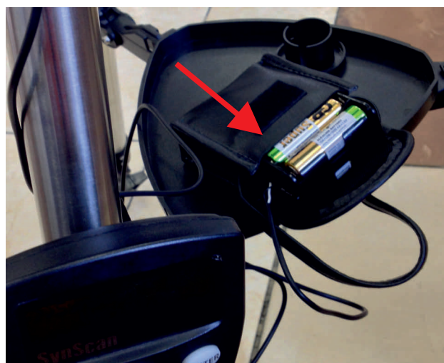
14. Battery box accepts eight AA batteries (purchased separately)
