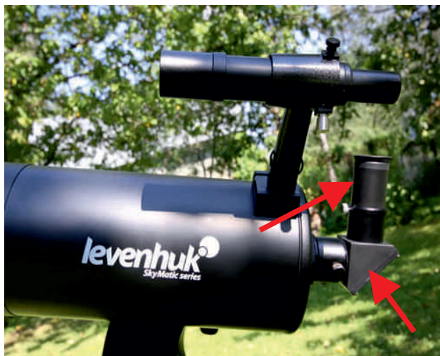
11. Fully assembled optical tube, with the diagonal mirror and an eyepiece
