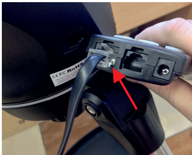
15. RJ-6 connector of the hand controller cable
