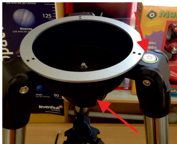
4. Tripod head without the mount. The clamping screw is in the center
