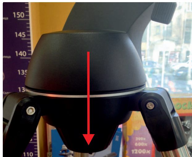
6. Clamping screw of the tripod head
