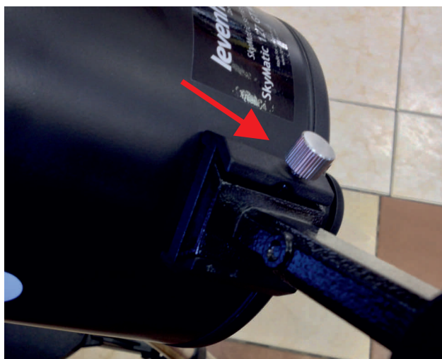
9. Tighten this thumbscrew to lock the finderscope mount in place
