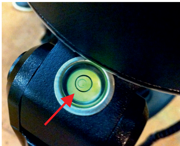
19. Spirit level (the bubble has to be within the center ring)
