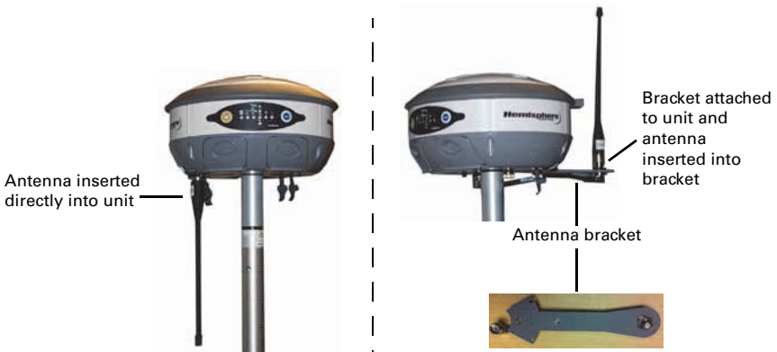
Figure 2-2: Antenna installation options
