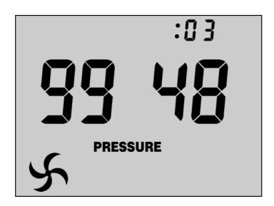
At the end of this period, the control system once again collects pressure data. The values recorded for attic pressure, both during fan operation and without, are compared to determine the amount of attic depressurization present. The result is then evaluated to determine the final status of the test.
