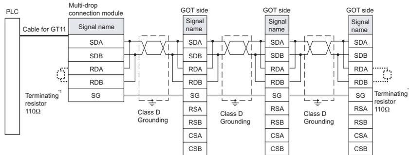
\*1 The terminating resistor 110 $\Omega$  is built in the multi-drop connection module and GOT (GT10,GT11).
