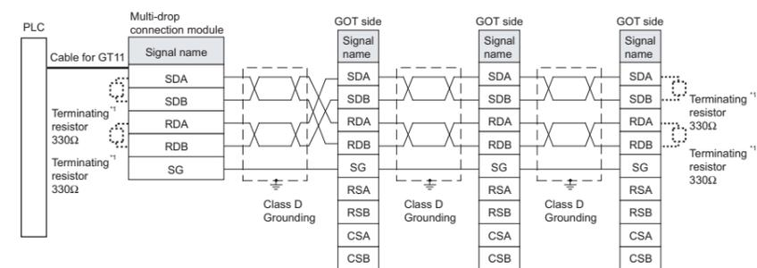
\*1 The terminating resistor 330Ω is built in the multi-drop connection module and GOT (GT10,GT11). Make sure to set the terminating resistor to both ends of the line. For GT15 or GT16, external wiring is required. Set the terminating resistor of the GOT that is not at the end of the line to "OPEN".
