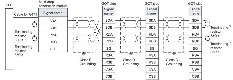
\*1 The terminating resistor 330 $\Omega$  is built in the multi-drop connection module and GOT (GT10,GT11).
