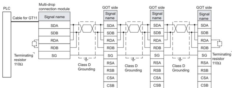
\*1 The terminating resistor 110Ω is built in the multi-drop connection module and GOT (GT10,GT11). Make sure to set the terminating resistor to both ends of the line. For GT15 or GT16, external wiring is required. Set the terminating resistor of the GOT that is not at the end of the line to "OPEN".
