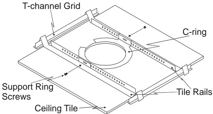
Figure 4: Mounting the Galil 6-C
