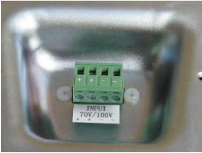
Figure 5: Plugging and Securing the Cable
