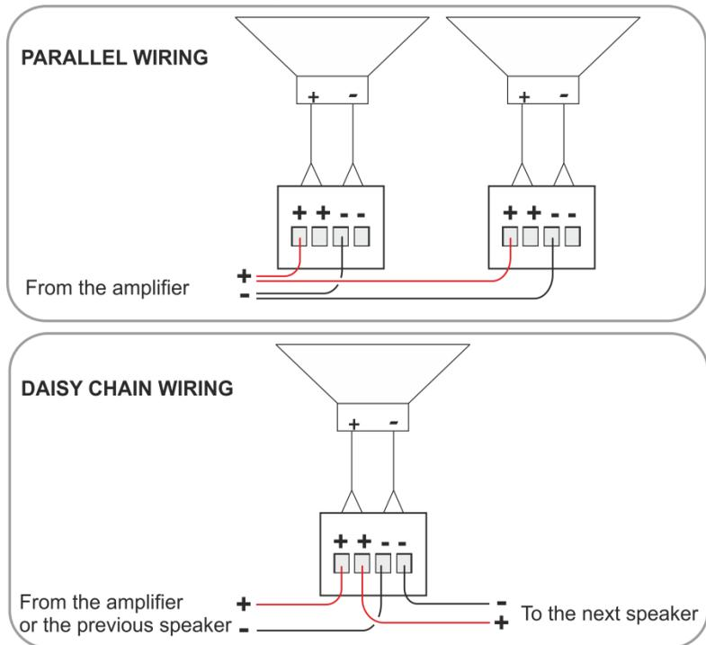
Figure 3: Galil 6-C Schematic Diagram
