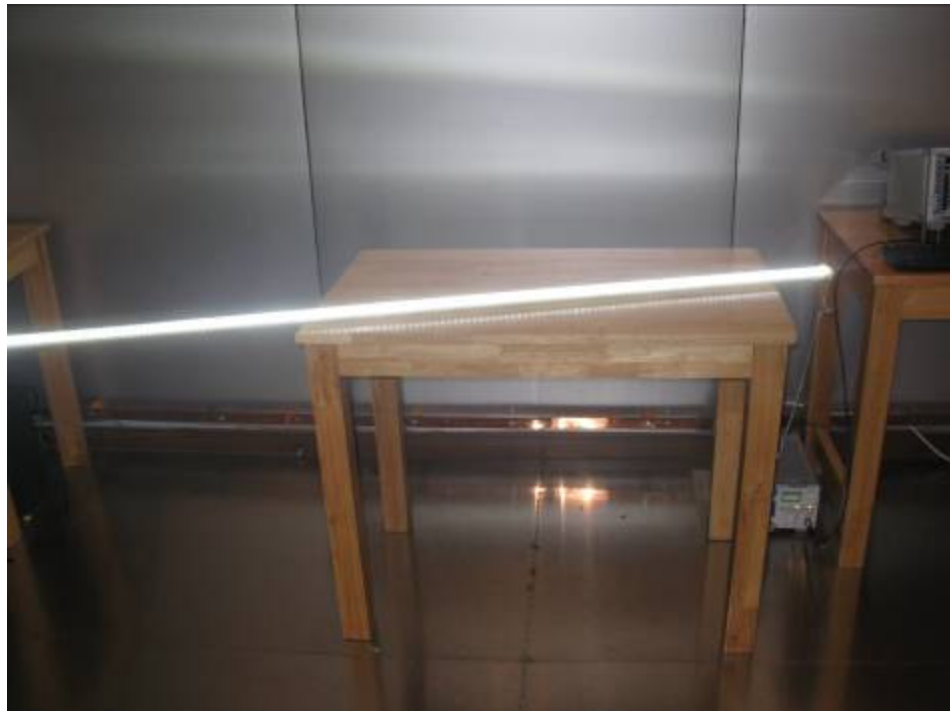
Figure 2 Conducted Emission test setup
