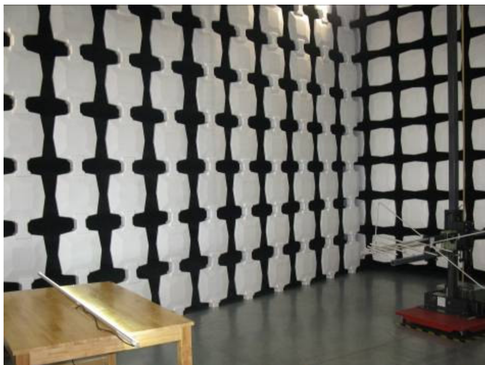
Figure 3 Radiated emission test setup
