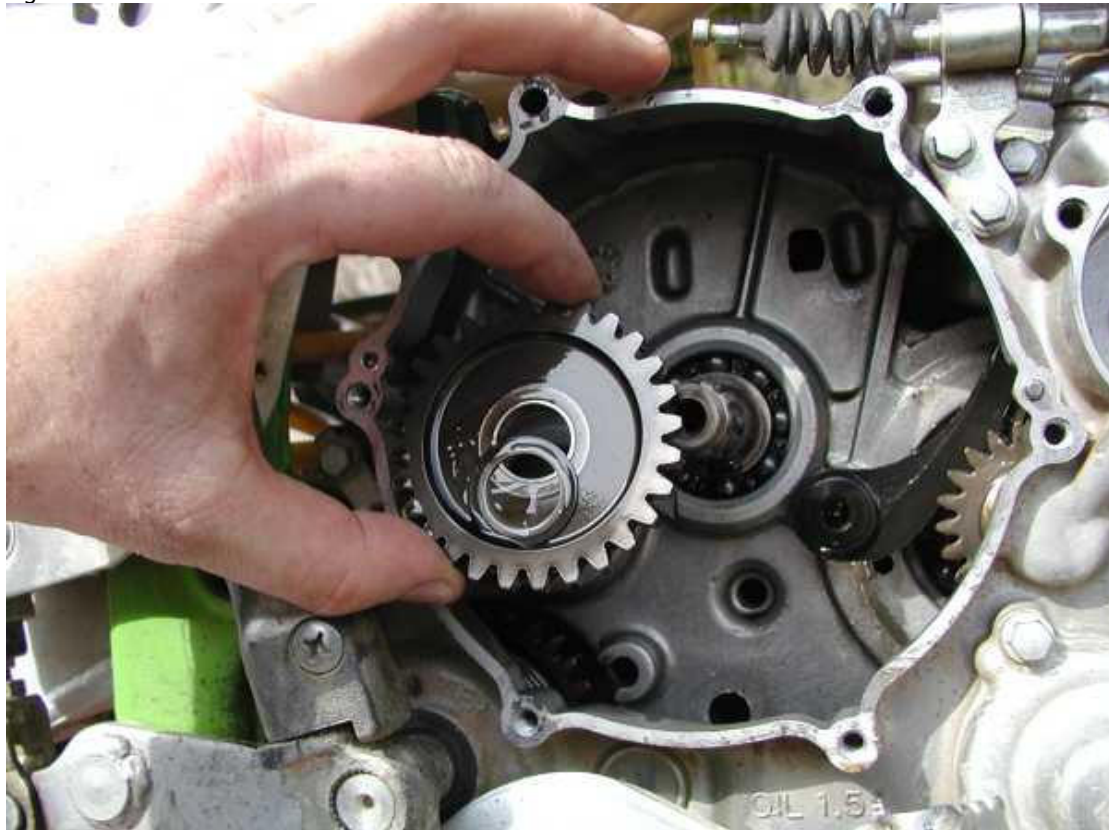
Figure 10: Note the Outer Shim Washer as I remove the Idler Gear.
