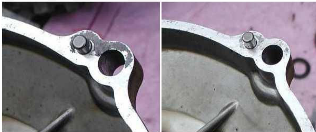
Figure 16: Cleaning the mating surface of the clutch cover and housing.
