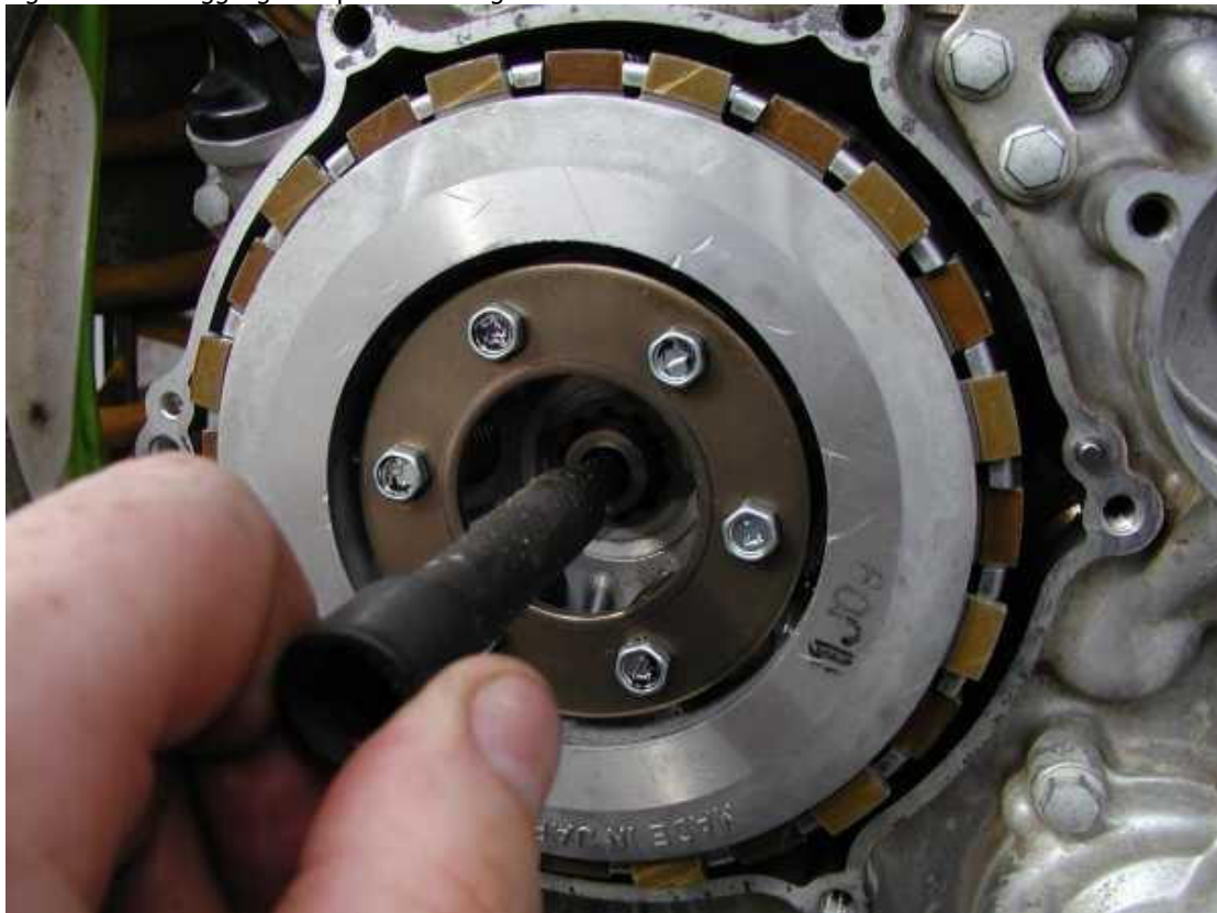
Figure 15: Me wiggling the splines into alignment
