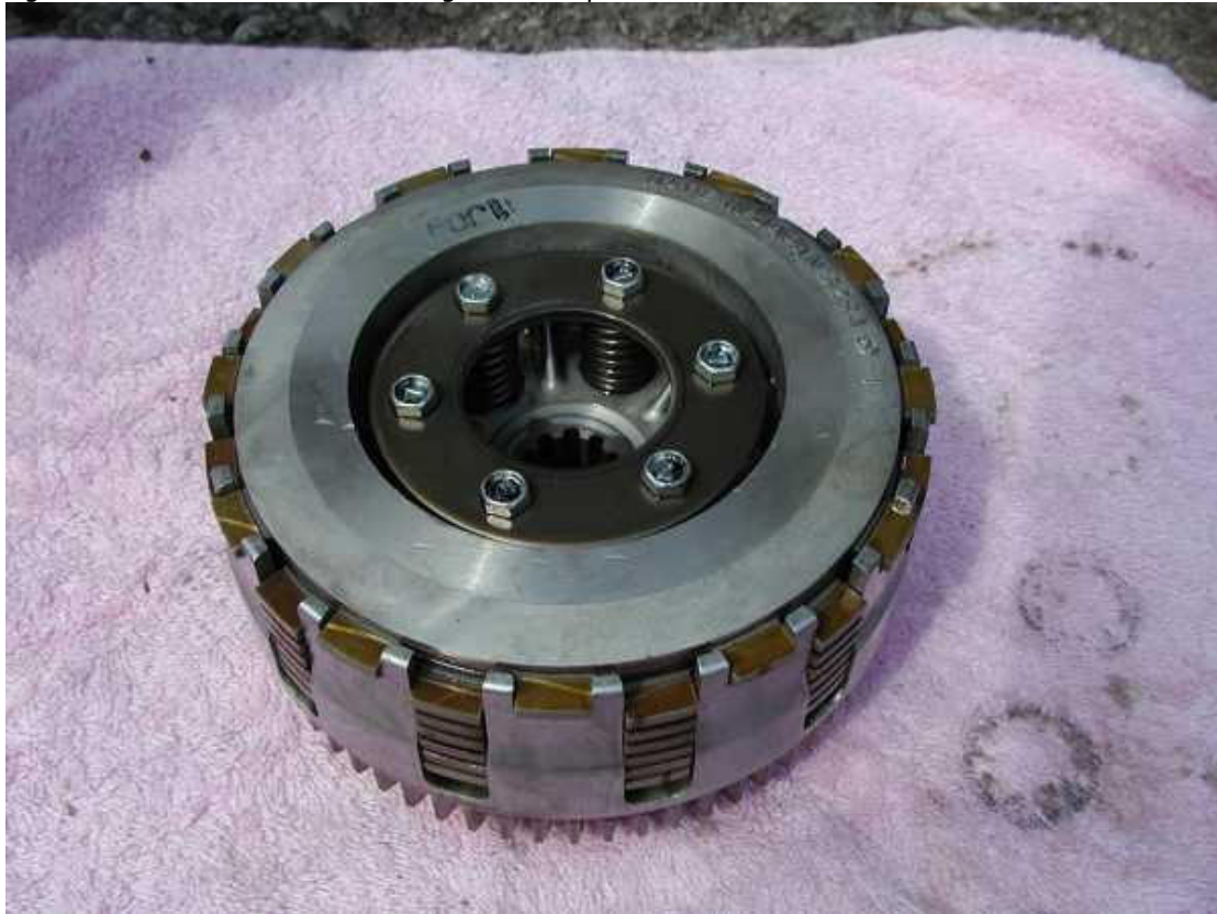
Figure 7: The Clutch Basket containing the clutch plate mechanism after removal.
