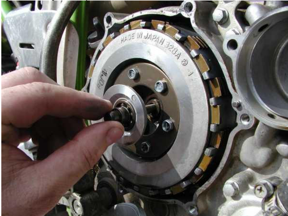
Figure 4: Removing the clutch pusher from the centre of the clutch.
