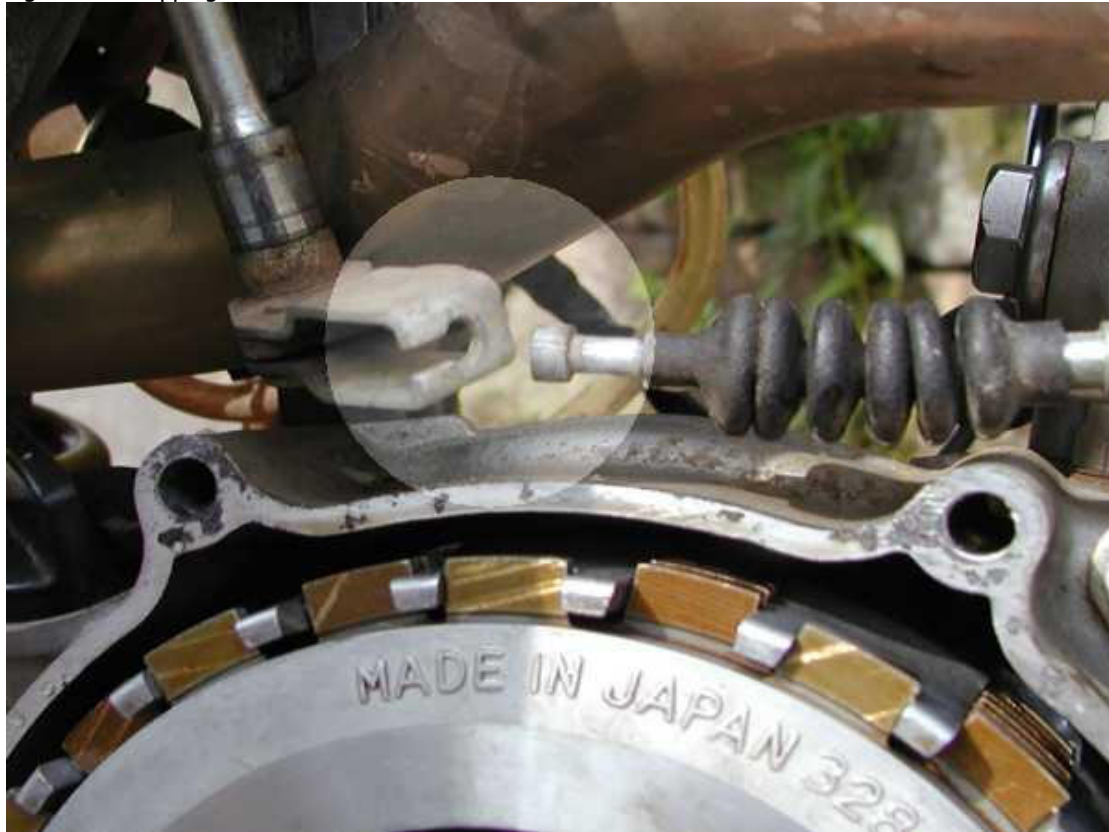
Figure 2: Unclipping the Clutch Cable.
