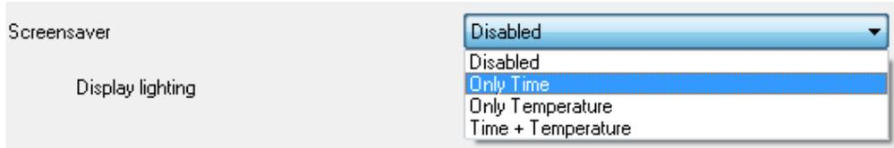
It is possible to configure the screensaver to only show the current **Time**, the current **Temperature** (selecting the desired measurement source: Internal temperature sensor or a external value, received by the "[General] Screensaver temperature" object) or **both** (alternatively every 5 seconds).
