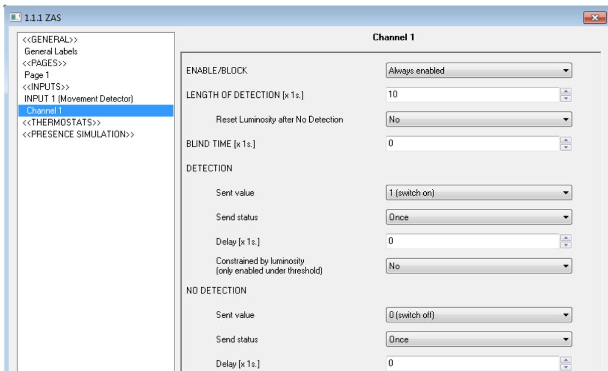
Figure 3.17. Channel configuration
