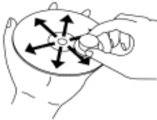
Wipe in the radial direction.
