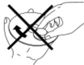
Do not wipe in the circumference direction.
