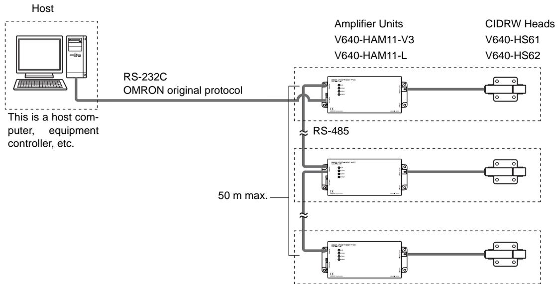
The Amplifier Units control the CIDRW Heads. Up to 31 Units can be connected.
