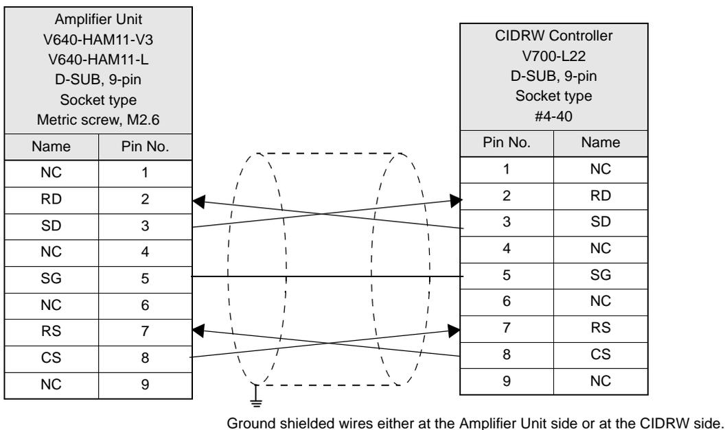
• **Wiring for Connection to a PC/AT Computer (9-pin Connector)**
