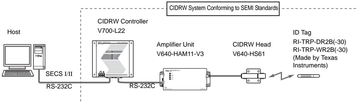
The V640-HS61 CIDRW Head can be connected to V640-HAM11-V3 Amplifier Units to communicate with ID Tags.
