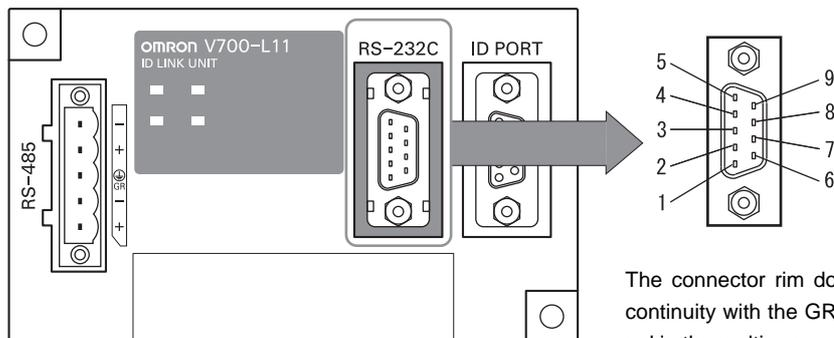
The connector rim does not have electrical continuity with the GR (frame ground) terminal in the multi-connection port.
