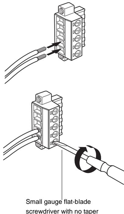
Small gauge flat-blade screwdriver with no taper
