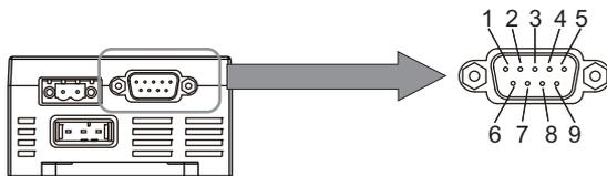
The connector rim has electrical continuity with the GR (frame ground) terminal in the dedicated power supply connector.
