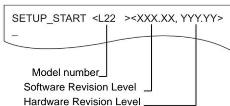
**Terminal Display When Parameter Setting Has Been Completed without Error**
