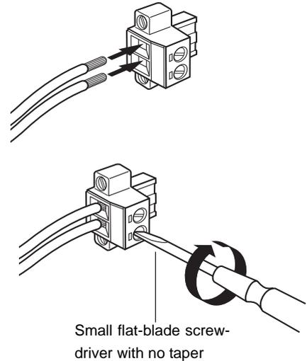
Small flat-blade screwdriver with no taper
