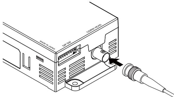
2. After inserting the connector fully home, turn the fixed part clockwise to lock it.
