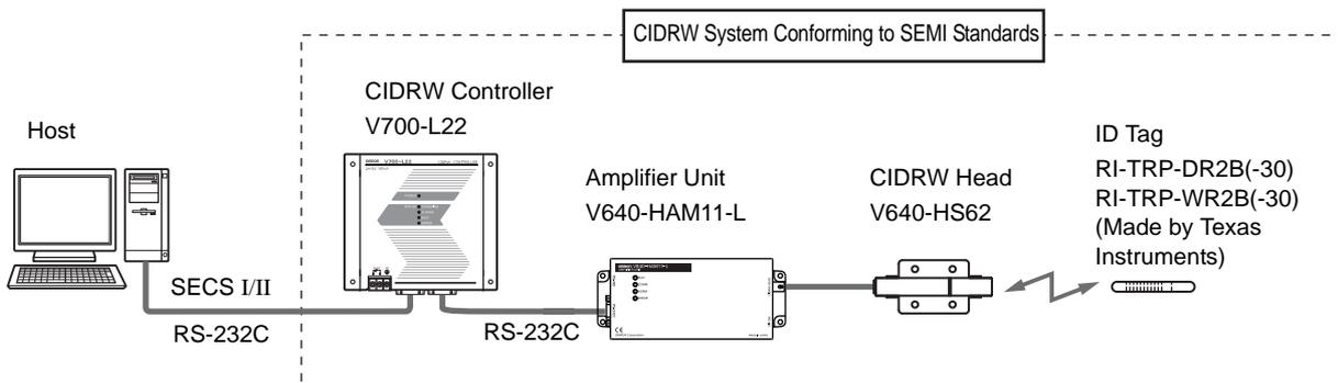
The V640-HS62 CIDRW Head can be connected to V640-HAM11-L Amplifier Units to communicate long-distance with ID Tags. The functions of the V640-HAM11-L Amplifier Unit are the same as the functions of the V640-HAM11-V3 Amplifier Unit.
