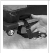
**1.** Attach the parking break strap to the back frame.
