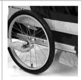
Pushing with your thumb over the black tip of the axle bolt, insert into desired hole on side of cab. Release the bolt and push until you hear it click. Pull on the wheel to ensure it is locked in place.
