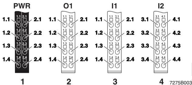
Figure 5 Terminal point assignment of the Inline connectors
