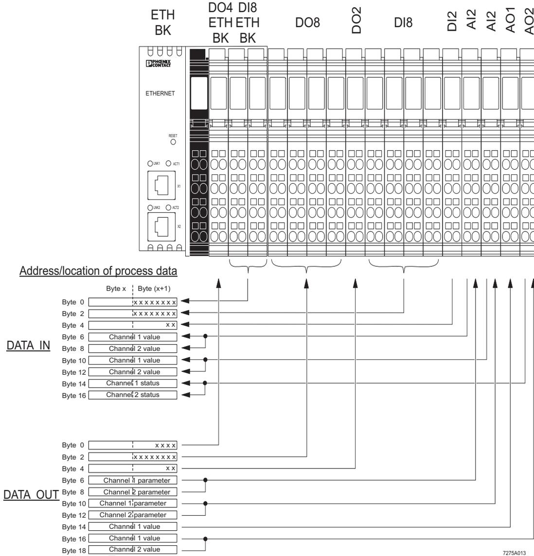
Figure 20 Assignment of process data
