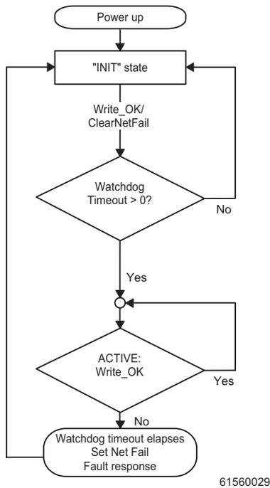
Figure 16 Status diagram of the process data watchdog
