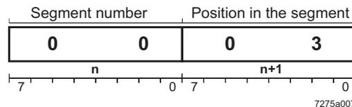
Figure 18 Contents of the local bus diagnostic parameter register (example)
