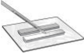
Fig 5. Wetting electrode wicks with electrode buffer.
