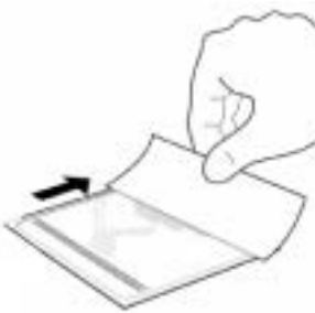
Fig 3. Dry the surface of the rehydrated gel with the edges of a gel drying board.
