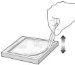
Fig 2. For even buffer distribution, carefully lift the opposite side of the film.
