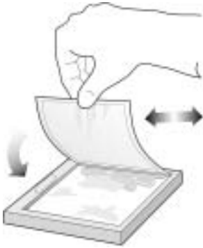
Fig 1. Lower the film with the gel surface downward into the rehydration buffer.
