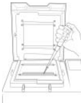
Fig 6. Loading samples with a pipette.
