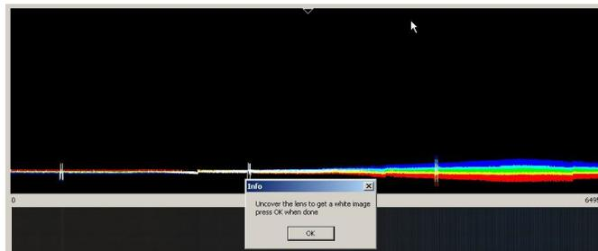
*Fig. 8 Sample signal after black offset calibration*
