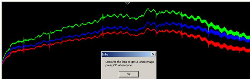
*Fig. 9 Sample signal before ADC gain calibration*
